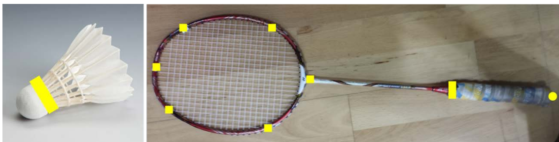
Figure 3. The marker and reflective tape attached to the racket and shuttlecock.
